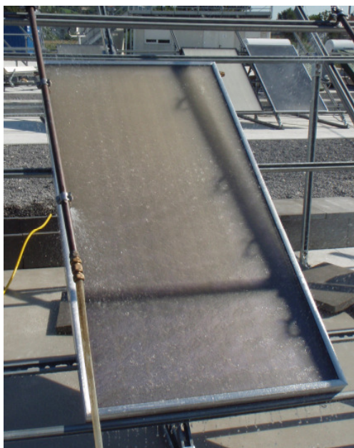
Fig. 3: rain penetration test
